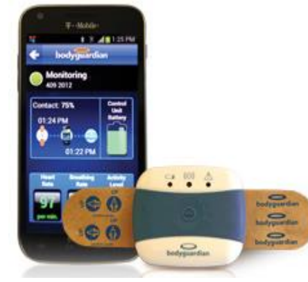
Preventice 's smart bandage constantly tracks cardiac ECG and rhythm monitoring
